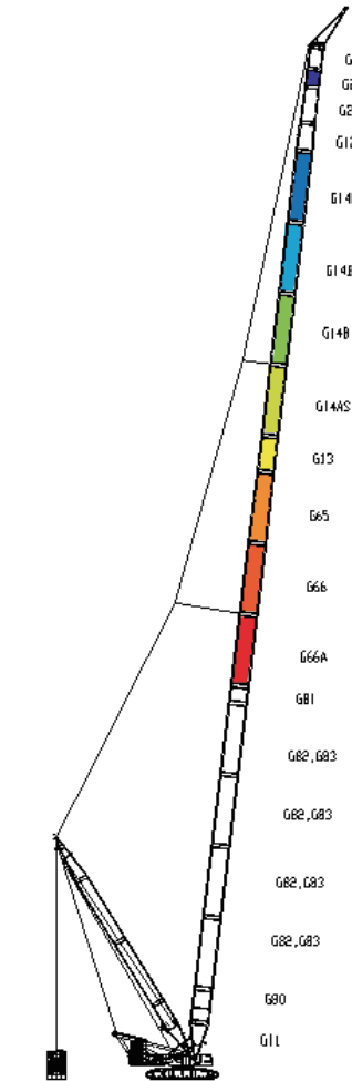
Superlift power boom booster + wind power lifting combination SLHSDB-2 (147m-171m+7m)
