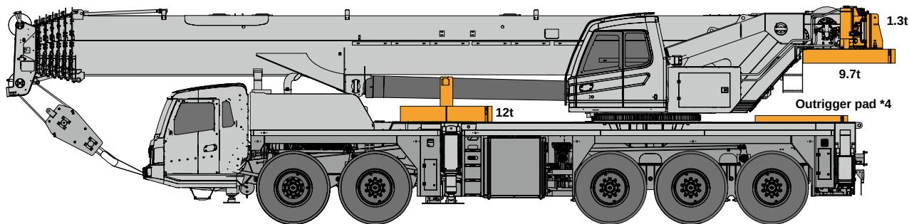
1.3t+9.7t+12t=23t, 4 outrigger pads are placed in rear section of frame
