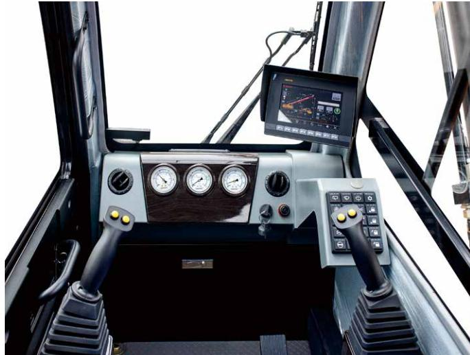
CAN BUS system: Controllers, displays, gauges, I/O modules, sensors, etc. are integrated in CAN Bus networking, fast-responsive.
